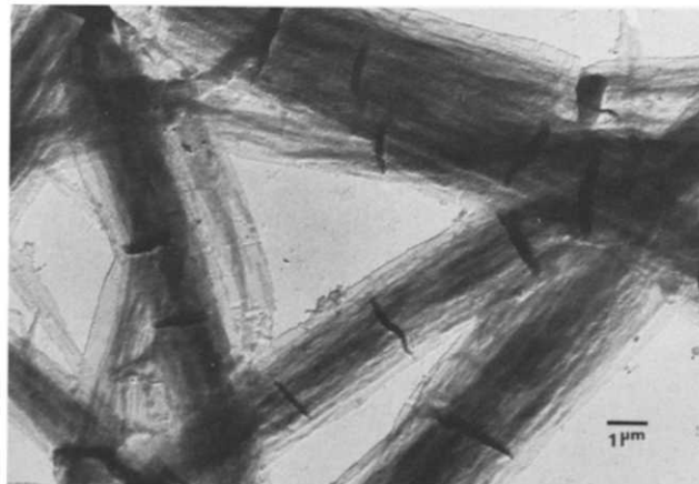
Figure 3 Electron micrograph of PBPP crystals obtained after quenching specimens from 180°C into liquid nitrogen, followed by heating to 120°C for 1 h and afterwards cooling to room temperature
